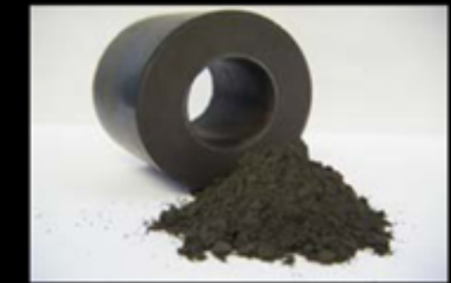
Dry molding compound (RD-396) with a SiC monolithic part fabricated from the same compound.
